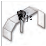
Retaining collar for mounting bracket with outside thread M10 x 1, bracket holes Ø10.5 or 13.5 mm incl. strain relief
